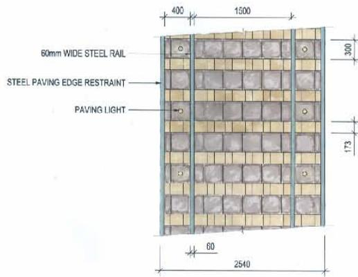
RAIL TRACK DETAILED CONCRETE PAVING
